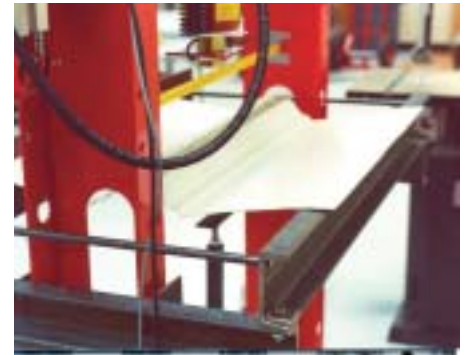
Small scale pull test to verify clip strength.
